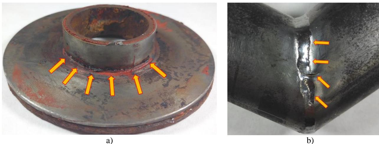
Fig. 1 Damaged welding joint of tantalum steam heating element.
