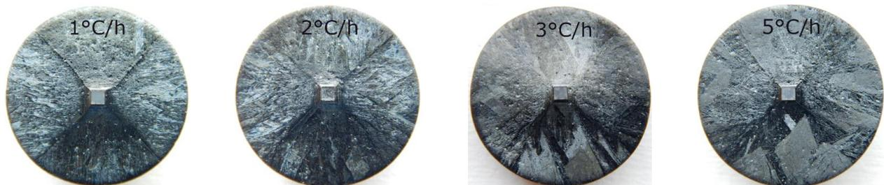
Fig. 1 Macrophotograph of the top of crystals prepared by different growth rates.
