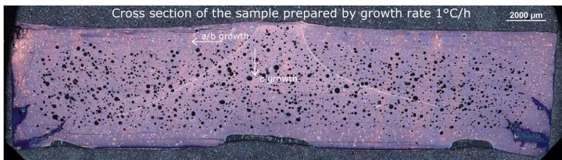
Fig. 2 Cross section of the sample prepared by growth rate 1 °C/h.
